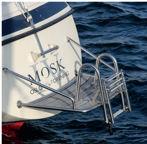
Bathing ladder with sturdy grips and universal fittings. Foot friendly steps.
